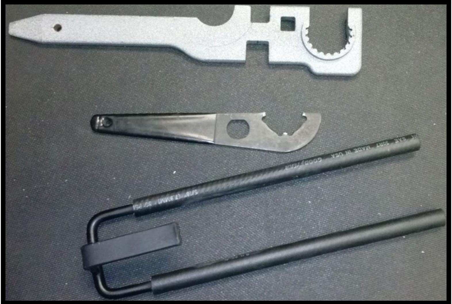
From top to bottom: AR combination wrench, castle nut spanner wrench, forearm tool
